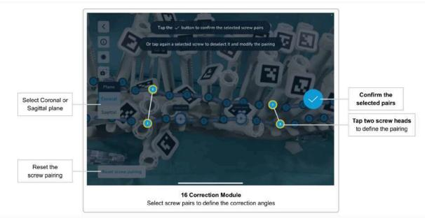
As a second step, you have to define one or multiple correction angles. You can apply correction angles on the coronal plane or on the sagittal plane, or on both simultaneously. To define a correction angle on the sagittal plane you have to select one screw pair, whereas on the coronal plane you have to select two screw pairs.
