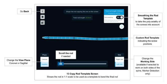
The *Copy Rod Template Screen* shows the shape of a custom-generated rod template on the screen in a 1-1 scale in sagittal and coronal view. This allows the surgeon to bend a custom rod according to the generated shape.
