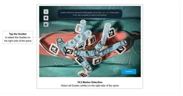
This step is only needed if you selected to work on both sides of the spine at the same time. It is skipped if you have selected to only scan one side of the spine at the time.
