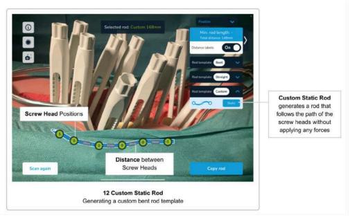
As described in the previous section, you can select any rod from the two categories straight and pre-bent rods. The third category of rods, called *Custom*, allows you to select a custom rod labeled as *static*.
