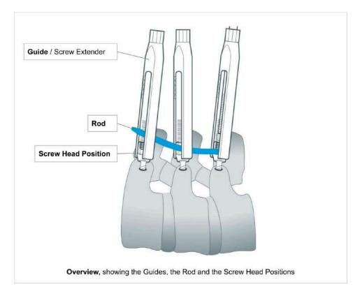
The guide is the screw head extension of the pedicle screw, also called Screw Extender. This extender helps the surgeon to perform rod reduction and manoeuvers during rod placement. We use the term "Guide" for the "Screw Extender" in this document.
