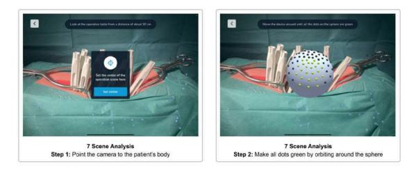
To start the scene analysis, tap the *Start* button. Now, point the device to the patient's body, so that the camera view shows the incision at a distance of about 50 cm. You will see a message if you are too close or too far away. Hit the *Confirm* button to set the center of the operation scene.
