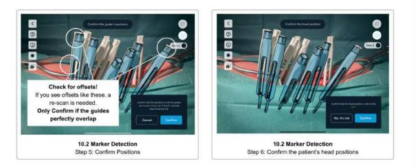
After having scanned all markers and tapped the *Finish scanning* (checkmark) button, again, visually check the virtual guides' positions and orientations. If you see offset guides, tap *Cancel* to go back and rescan offset guides. Only if all guides are perfectly overlapping the physical guides, tap *Confirm* to finish the scanning process.
