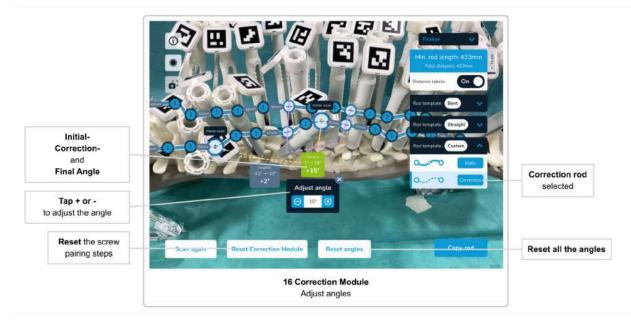
After selecting and confirming the screw pairing in the previous steps, you can see the angles between the predefined pairs.
