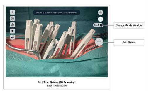
Start scanning the first guide by tapping the *Add Guide* button. Make sure that the correct version of the guide is selected by checking the *Guide Version Selection* toggle.
