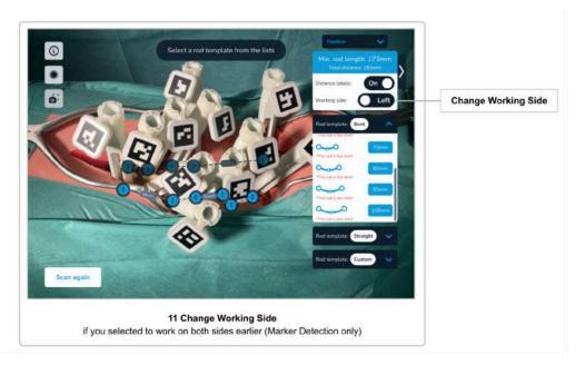
When using the Marker Detection scanning method, you have the option to scan both sides of the spine simultaneously. Select the option either in the dialogue that appears when selecting the Marker Detection scanning method or on the *Confirmation Overview* screen.
