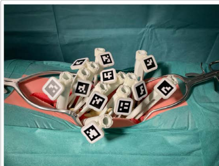
10.2 Scan Guides (Marker Detection) Place the markers to avoid occlusion by other markers
