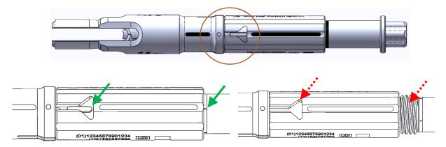
Left OK: sunk key engaged in racetrack, marking is flush.
